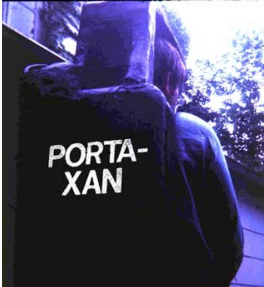
This wearable computer mockup is large and clumsy, about the size of a briefcase, with hooks over the shoulders and what was meant to look like a CRT (actually in the mockup it was a big flashlight) perched just on Dan's left shoulder. In front of his face (not visible) is a piece of plexiglas, representing a semi-transparent reflector for looking back at the CRT while you also look forward at the world.
