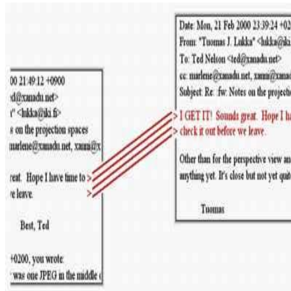
Figure 21. Simulated email viewer showing original context of a transclusion (rather than the usual disconnected quote). Customary inpointing angle brackets on the right indicate the transcluded material; outpointing on the left, they indicate the source.
